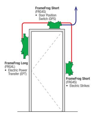
Conduit from FrameFrogs to the ceiling Conduit connecting FrameFrogs within frame
