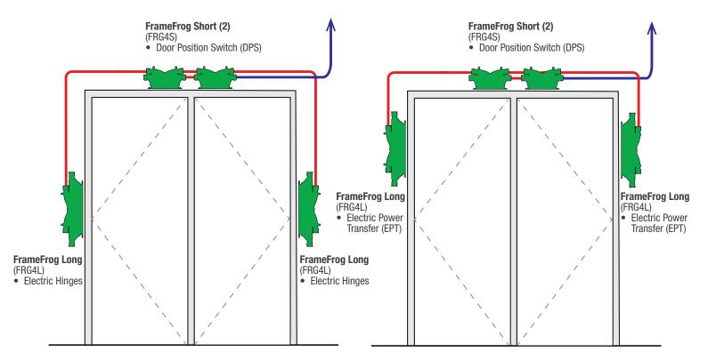
Conduit from FrameFrogs to the ceiling Conduit connecting FrameFrogs within frame
