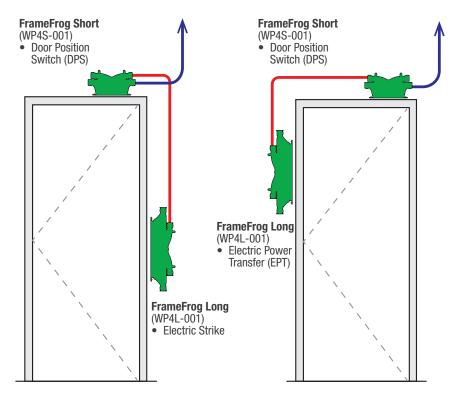
Conduit from FrameFrogs to the ceiling Conduit connecting FrameFrogs within frame
